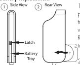
1. Using a small flat narrow object, push latch down towards battery tray while gently prying the tray outwards from both ends until released. Remove the tray from the remote constrol housing.
